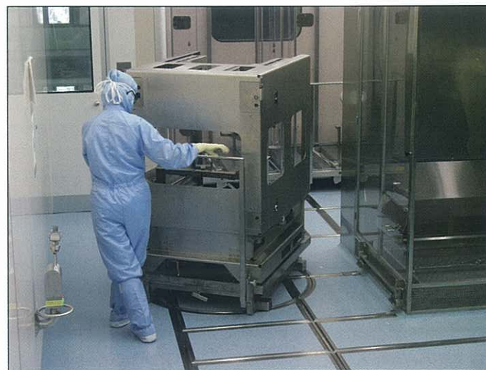
Transfer on rails of the chassis at the end of the campaign (without BPT).
