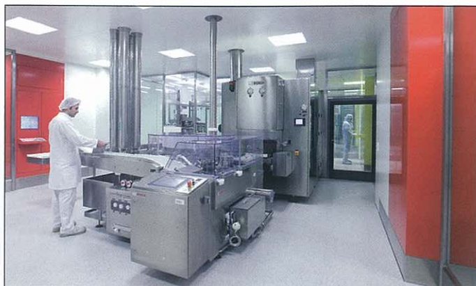
Setting the machines up in a u-shape reduces the space required in the highest cleanroom class and increases the employees' productivity.
