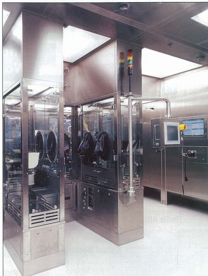
Glove ports for the syringe line that is integrated into the cleanroom wall; human machine interface (HMI) displays process and environmental data for operators inside the cleanroom.
