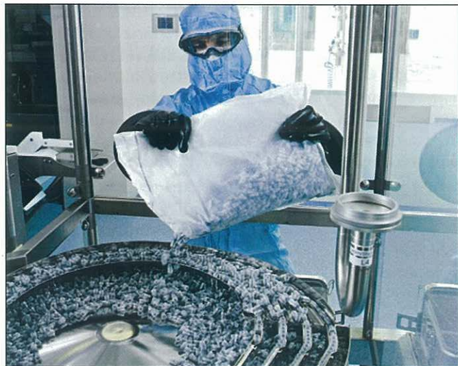
Aseptic intervention via gloves in RABS Technology.
