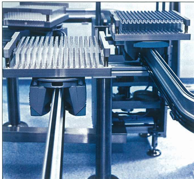
Automatic shuttle transportation system in cleanrooms.
