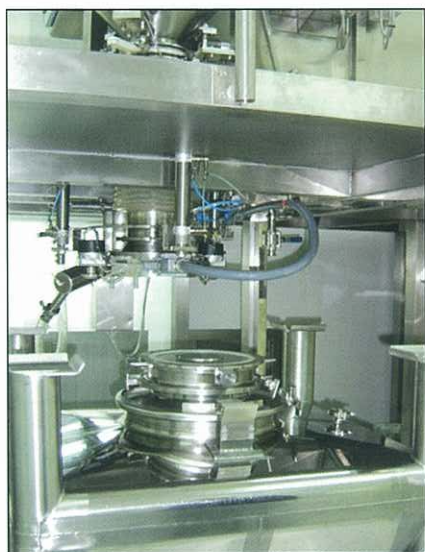
IBC container ready to be joined to the isolation valve.
