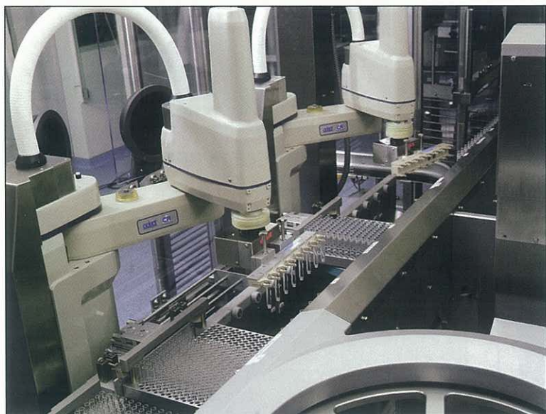
Automatic loading of transport magazines.
