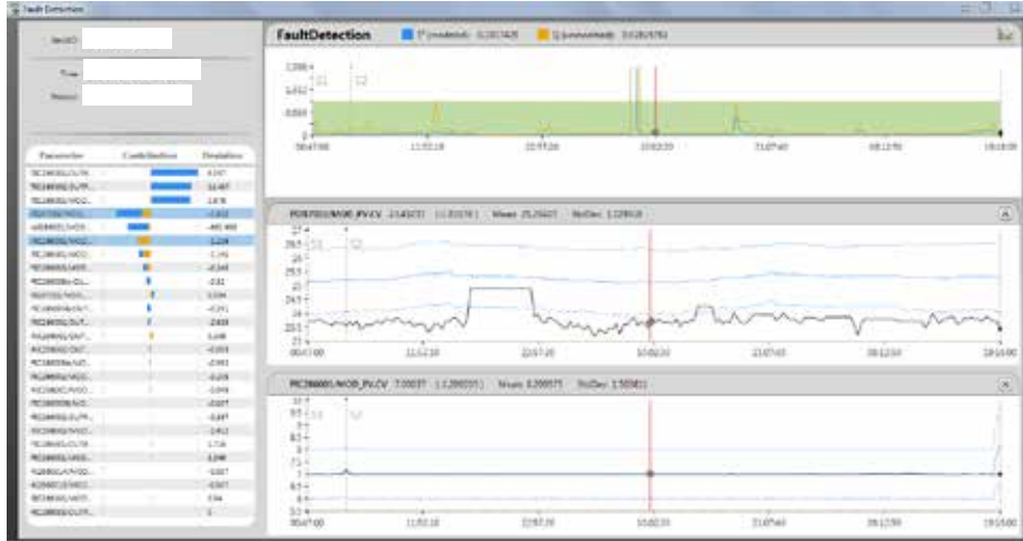
Figure 6: An example of a golden batch profile implementation through MVDA modeling.
